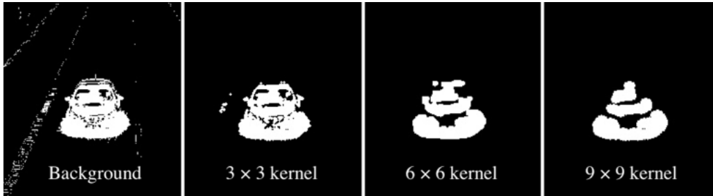
Figure 3.2: Background with morphology using different kernel sizes.
