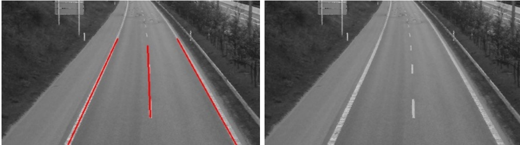
Figure 3.3: Example of detected lines (left) on a road image (right).
