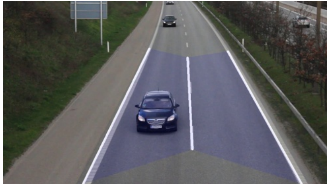
Figure 3.4: Example of lanes detected on a two-lane highway.
