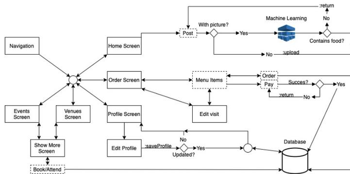
Figure 3: Diagram of the different screens and how they communicate
