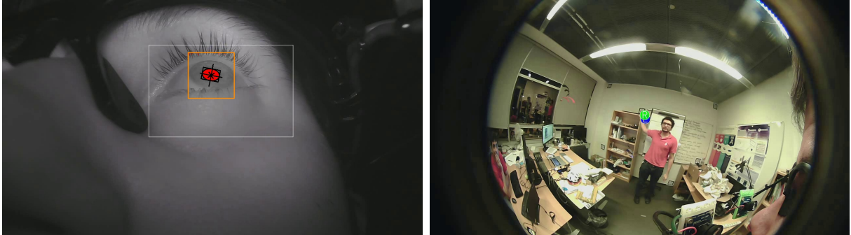
Figure 4: An example of synchronized images captured by a head-mounted eye tracker. ( left ) the user's eye captured by the eye camera; and ( right ) the scene image that represents the user's field of view.
