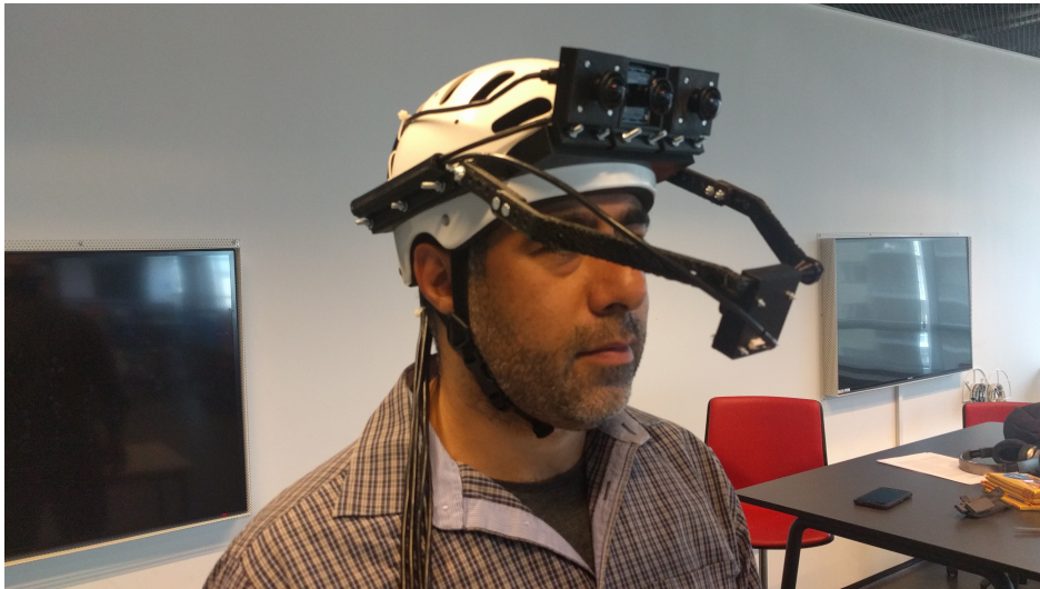
Figure 22: The head-mounted eye tracker used for the parallax error experiment. This device had three scene cameras, one eye camera to capture the binocular information from the user (built in May 2017).
