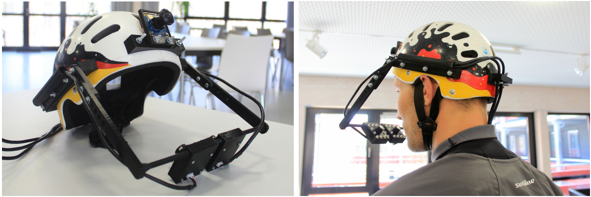
Figure 68: A head-mounted eye tracker prototype built with off-the-shelf hardware in a kayak helmet.
