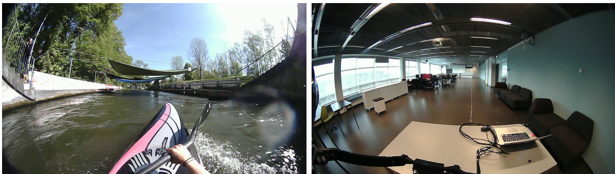
Figure 25: Two different images captured from a scene camera using a M12 eye-fish lens of 1.21mm (focal length) and f/2.0 (aperture). This lens has an angle of view of 220^\circ and it covers the entire subject's field of view. It is also possible to see a small region even behind the subjects. Cameras that use eye-fish lenses with a wide angle of view, capture the environment like a sphere.
